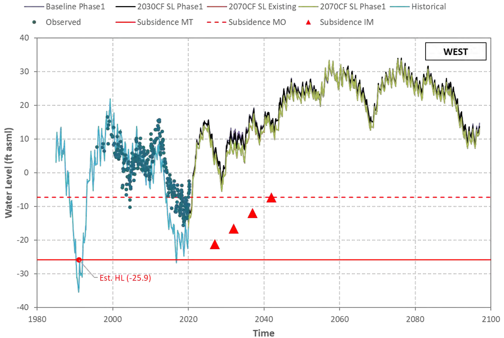
Figure I-14 Hueneme Aquifer - Simulated/Observed Water Level (Well 02N23W15J01S).
