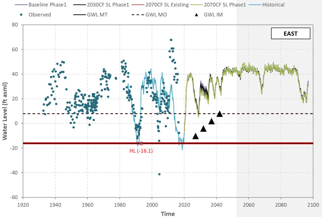
Figure H-16 Mugu Aquifer - Simulated/Observed Water Level (Well 02N22W07M02S)
