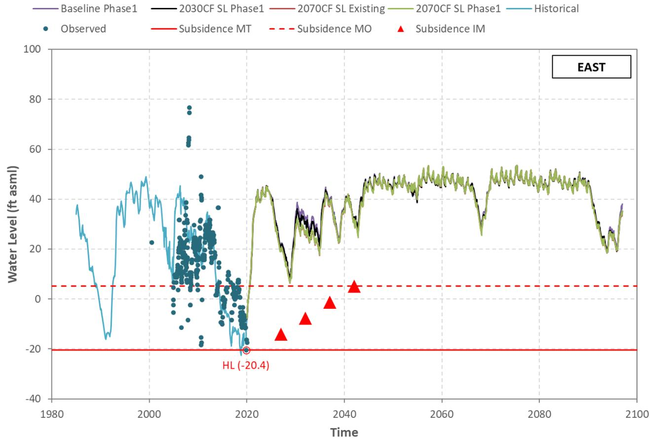
Figure I-16 Mugu Aquifer - Simulated/Observed Water Level (Well 02N22W08G01S).
