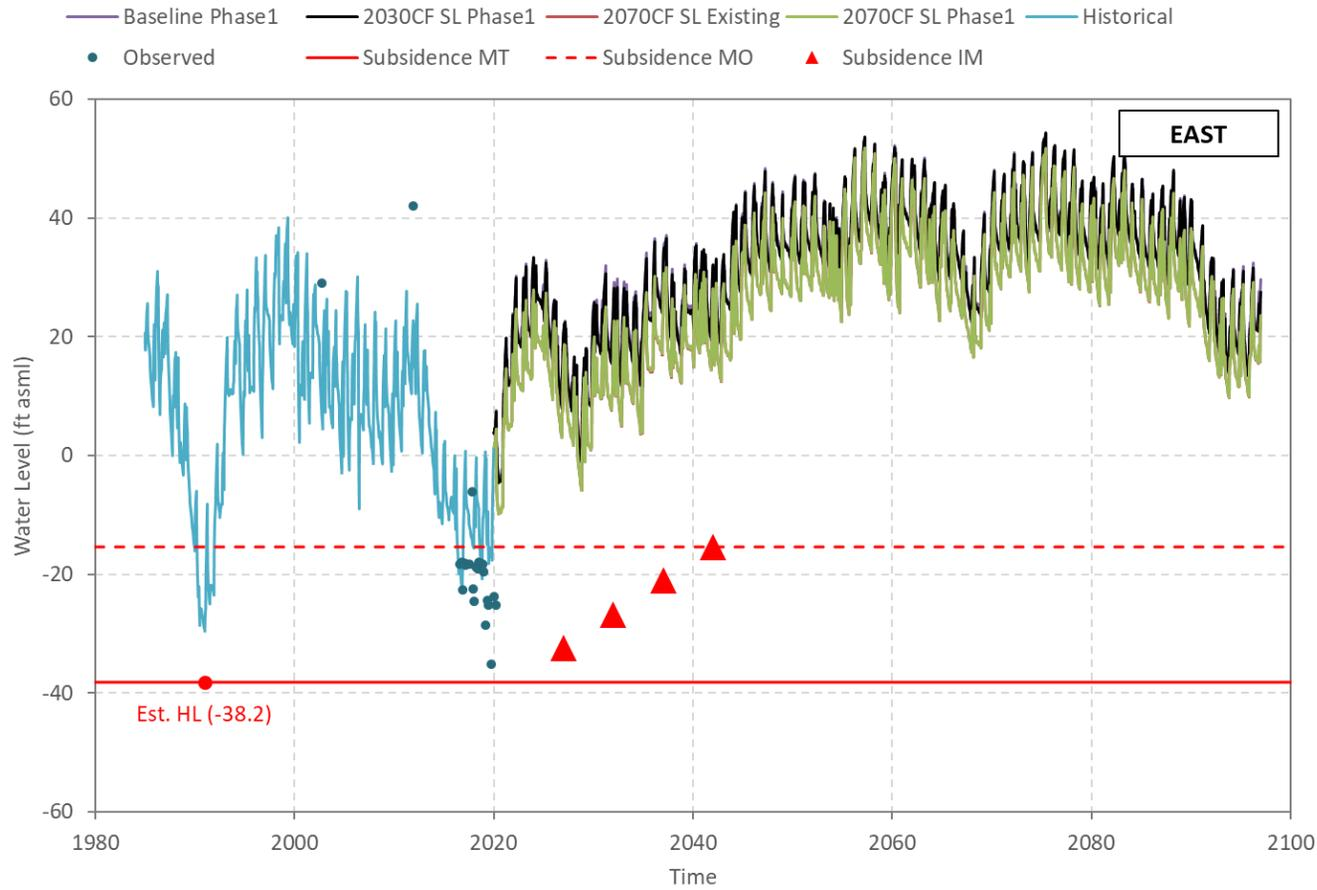
**Figure 1-6 Hueneme Aquifer - Simulated/Observed Water Level (Well 02N22W10N03S).**
