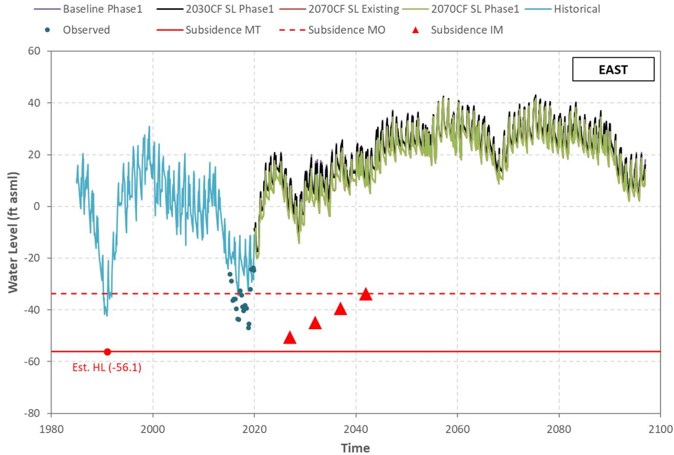
**Figure I-7 Hueneme Aquifer - Simulated/Observed Water Level (Well 02N22W16K01S).**
