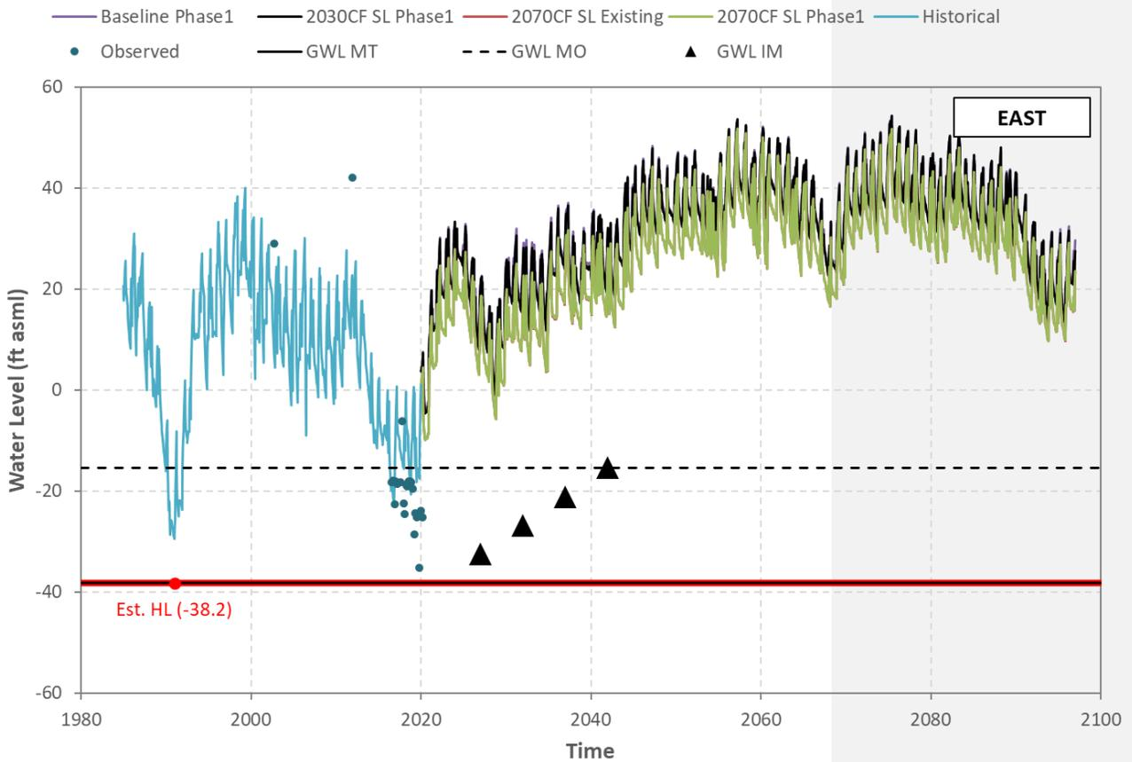
**Figure H-5 Hueneme Aquifer - Simulated/Observed Water Level (Well 02N22W16K01S)**
