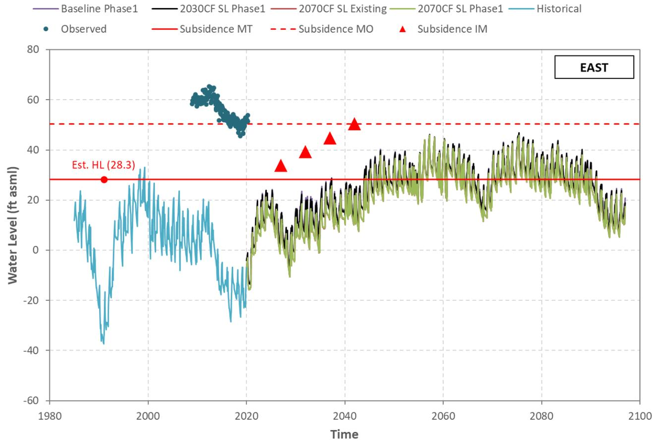
**Figure I-4 Hueneme Aquifer - Simulated/Observed Water Level (Well 02N22W09L03S).**
