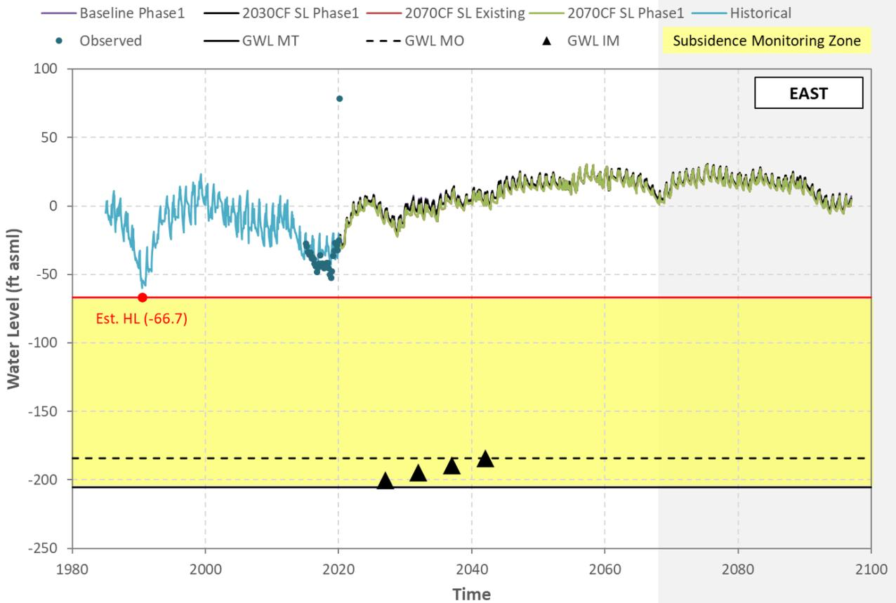
**Figure H-7 Hueneme Aquifer - Simulated/Observed Water Level (Well 02N22W07M01S)**
