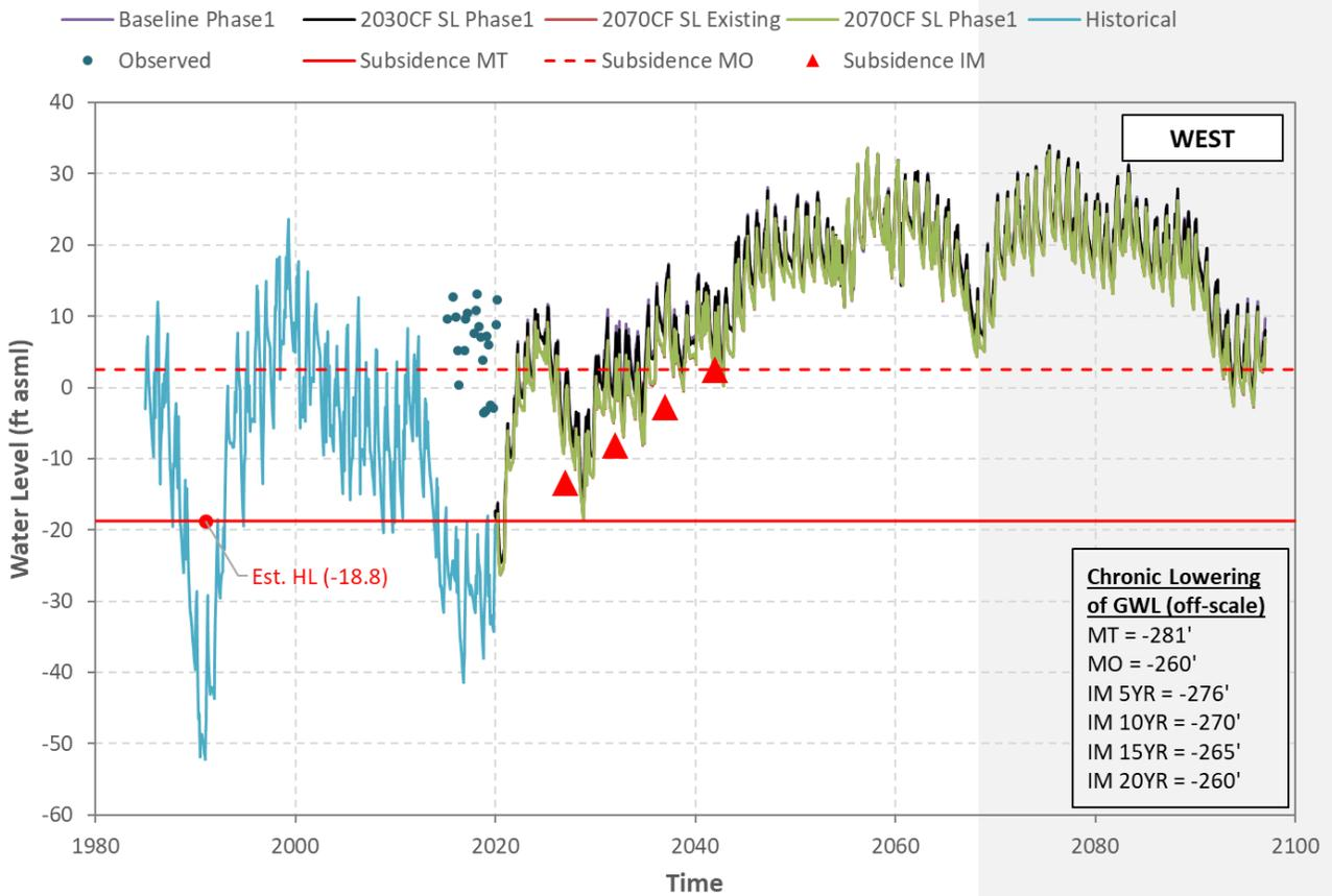
**Figure H-9 Hueneme Aquifer - Simulated/Observed Water Level (Well 02N22W20E01S)**
