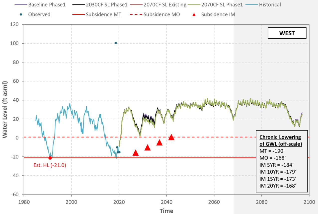
**Figure H-18 Mugu Aquifer - Simulated/Observed Water Level (Well 02N22W19M04S)**
