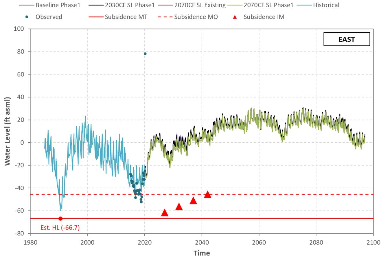
**Figure I-8 Hueneme Aquifer - Simulated/Observed Water Level (Well 02N22W17Q05S).**
