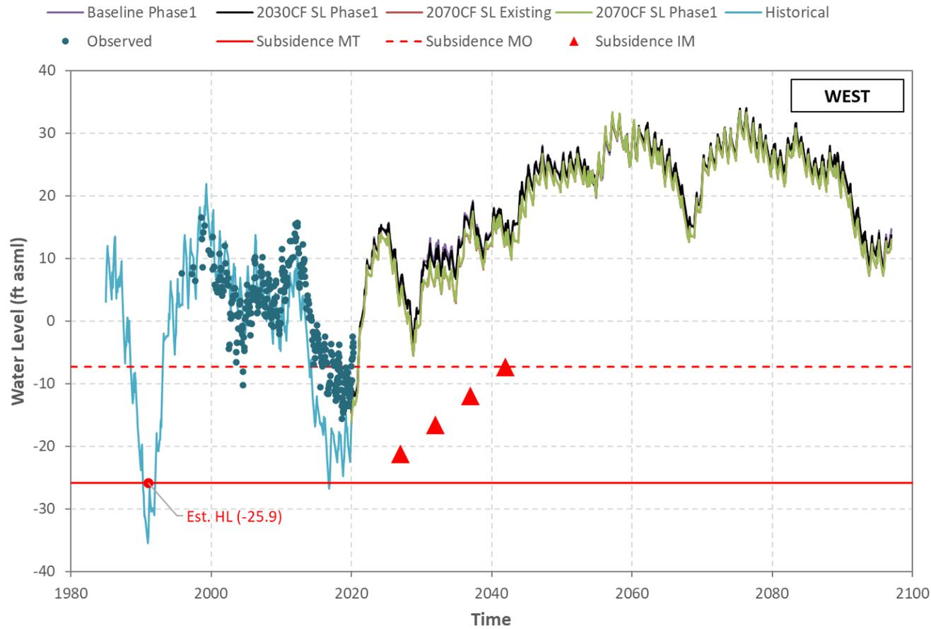
**Figure I-14 Hueneme Aquifer - Simulated/Observed Water Level (Well 02N23W15J01S).**
