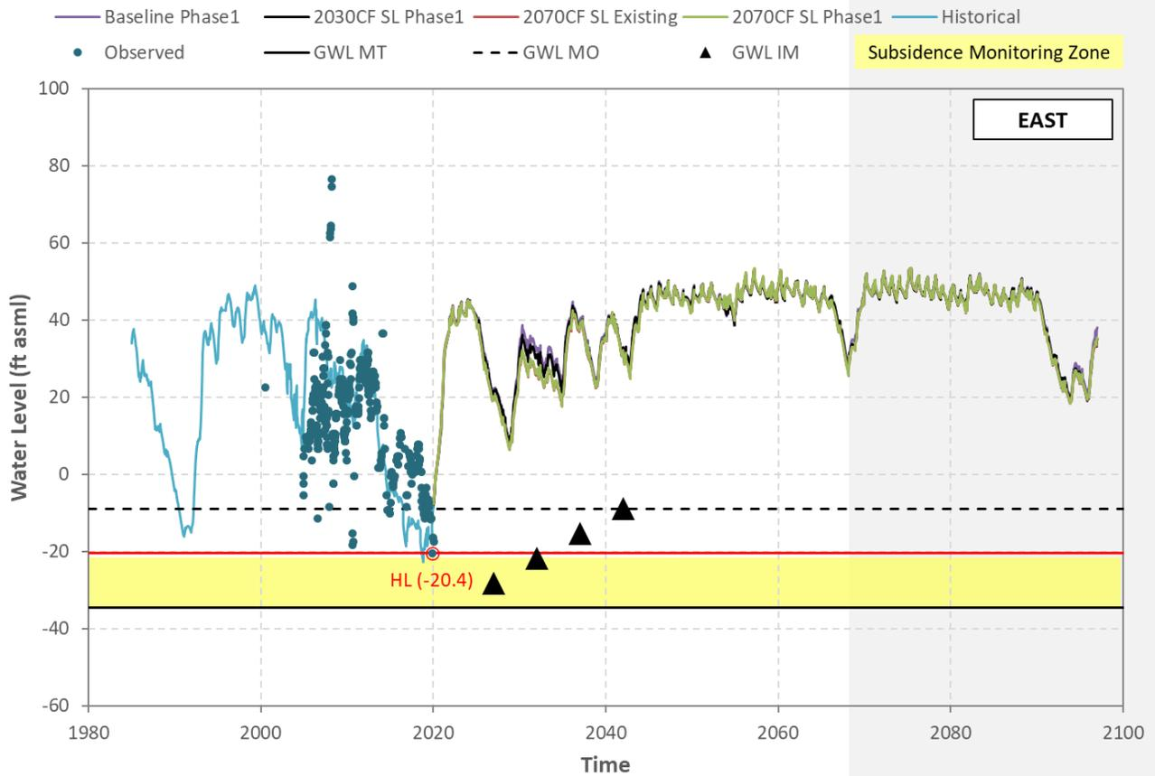
Figure H-15 Mugu Aquifer - Simulated/Observed Water Level (Well 02N22W08P01S)
