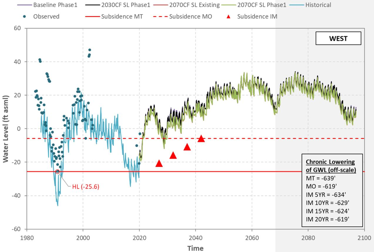
**Figure H-12 Hueneme Aquifer - Simulated/Observed Water Level (Well 02N23W15J01S)**
