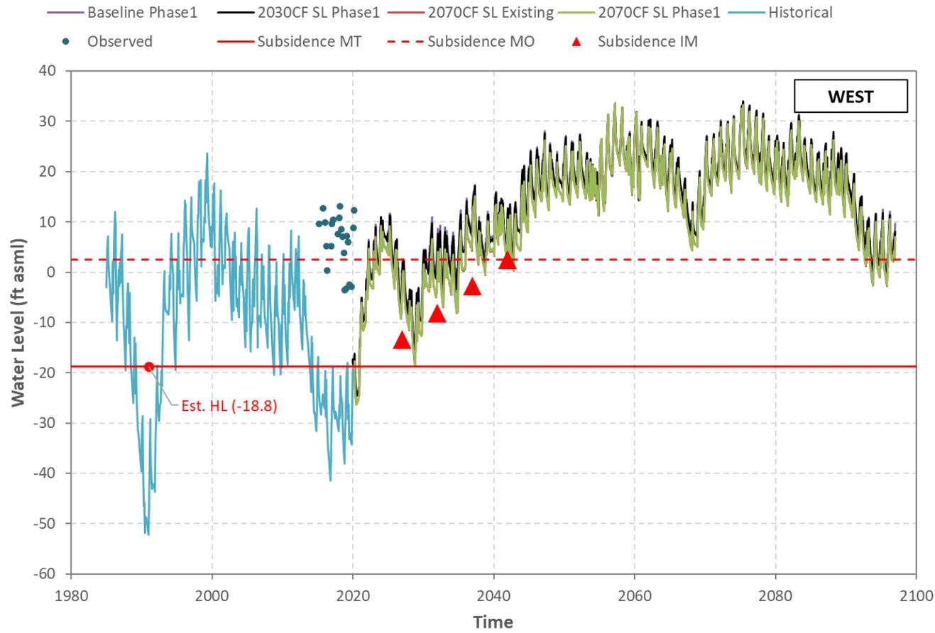
**Figure I-10 Hueneme Aquifer - Simulated/Observed Water Level (Well 02N22W17M02S).**
