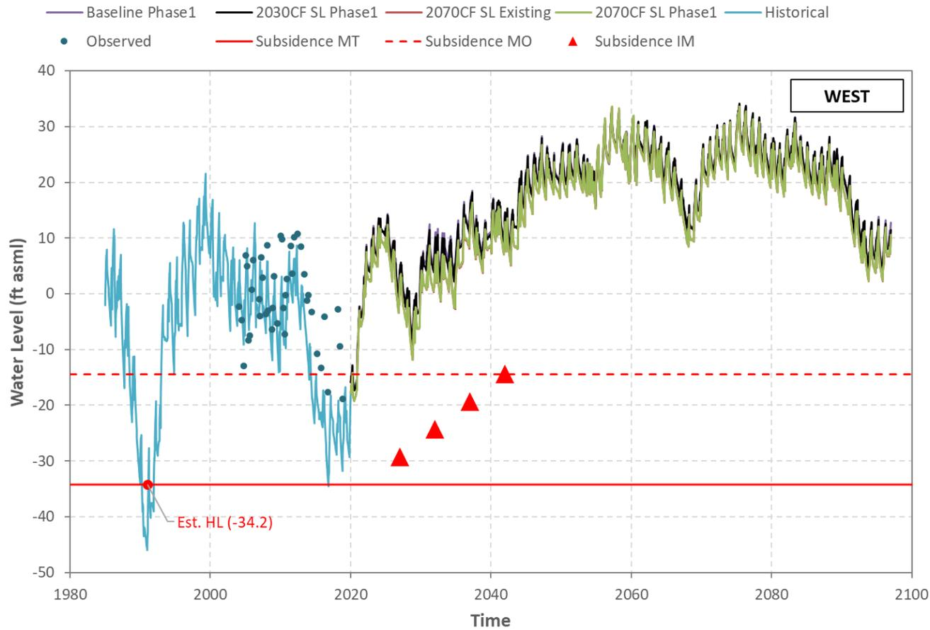
Figure I-12 Hueneme Aquifer - Simulated/Observed Water Level (Well 02N23W13K03S).
