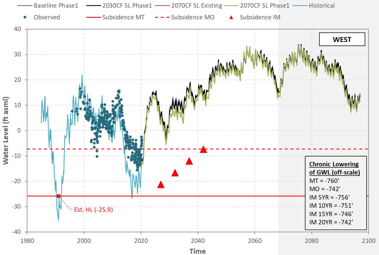
Figure H-13 Hueneme Aquifer - Simulated/Observed Water Level (Well 02N23W24G01S)
