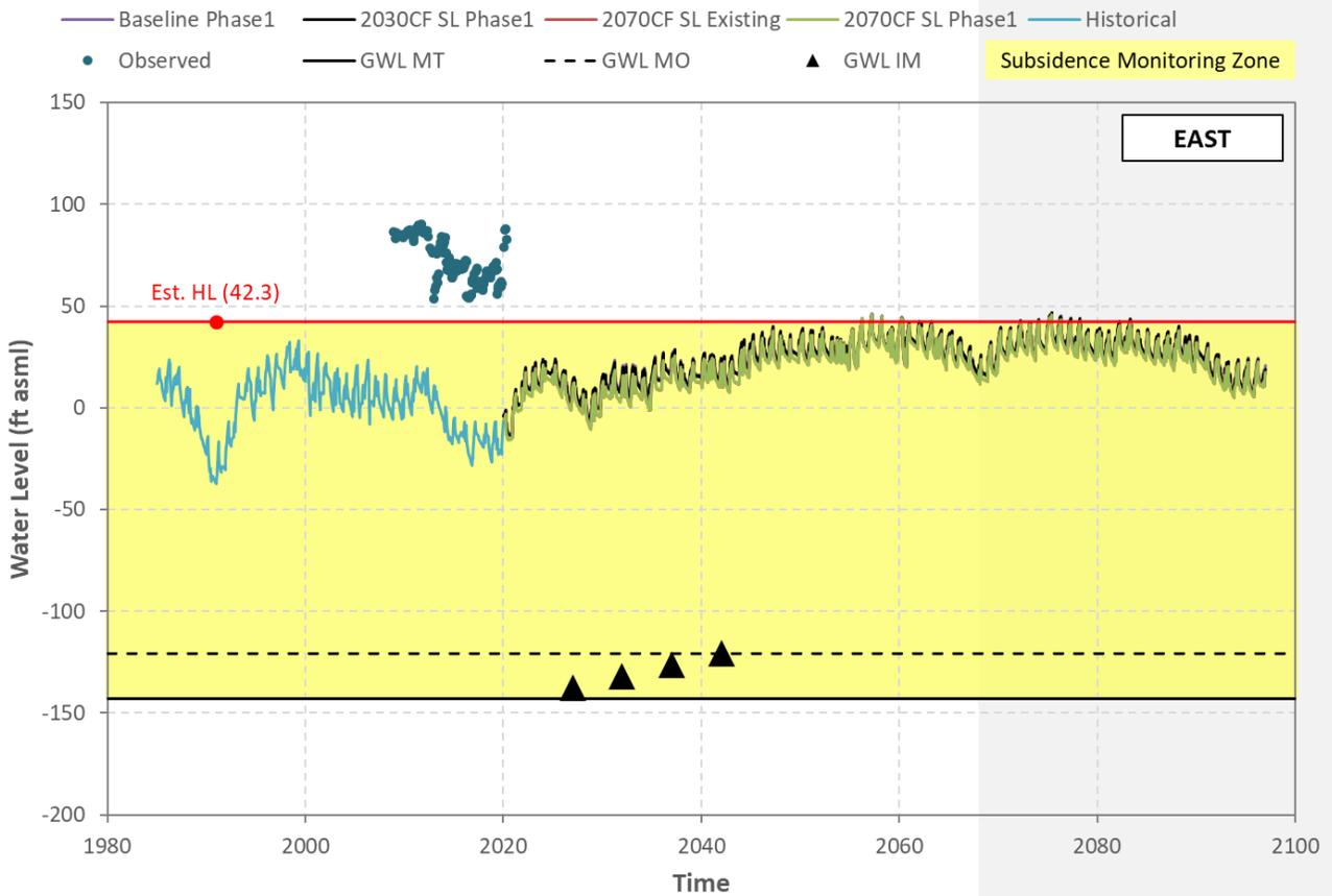
**Figure H-4 Hueneme Aquifer - Simulated/Observed Water Level (Well 02N22W10N03S)**
