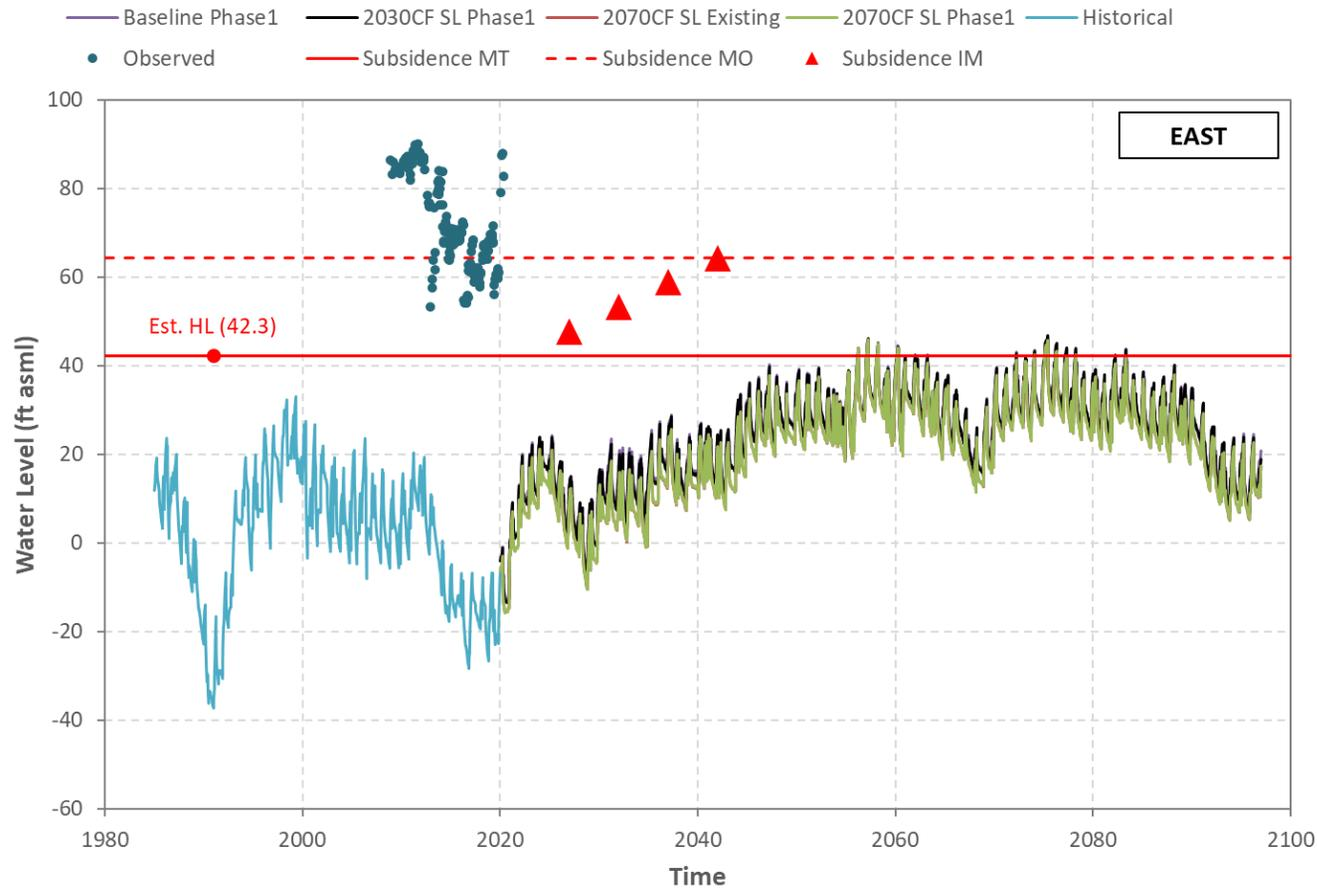
**Figure I-5 Hueneme Aquifer - Simulated/Observed Water Level (Well 02N22W09L04S).**
