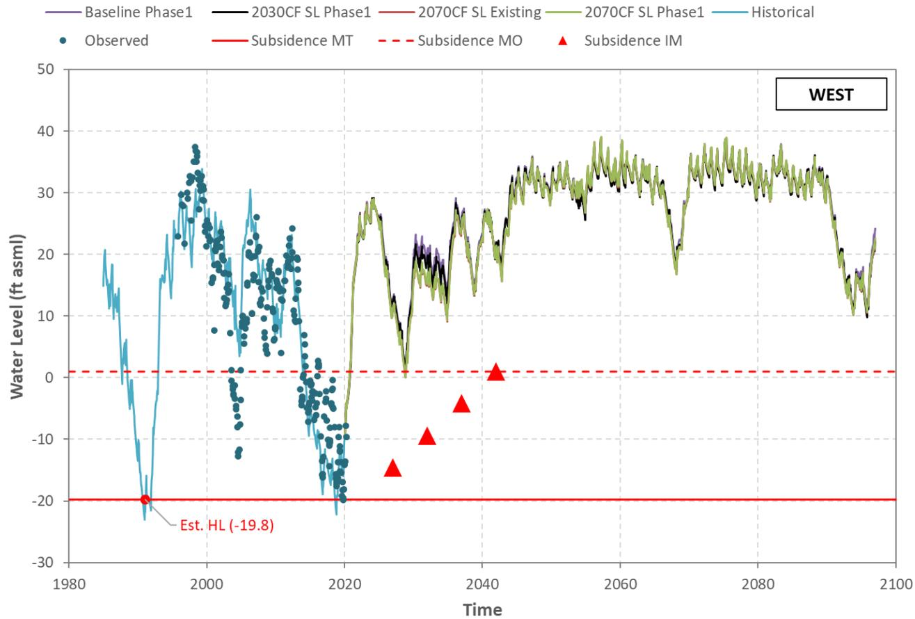
**Figure I-18 Mugu Aquifer - Simulated/Observed Water Level (Well 02N22W07M02S).**
