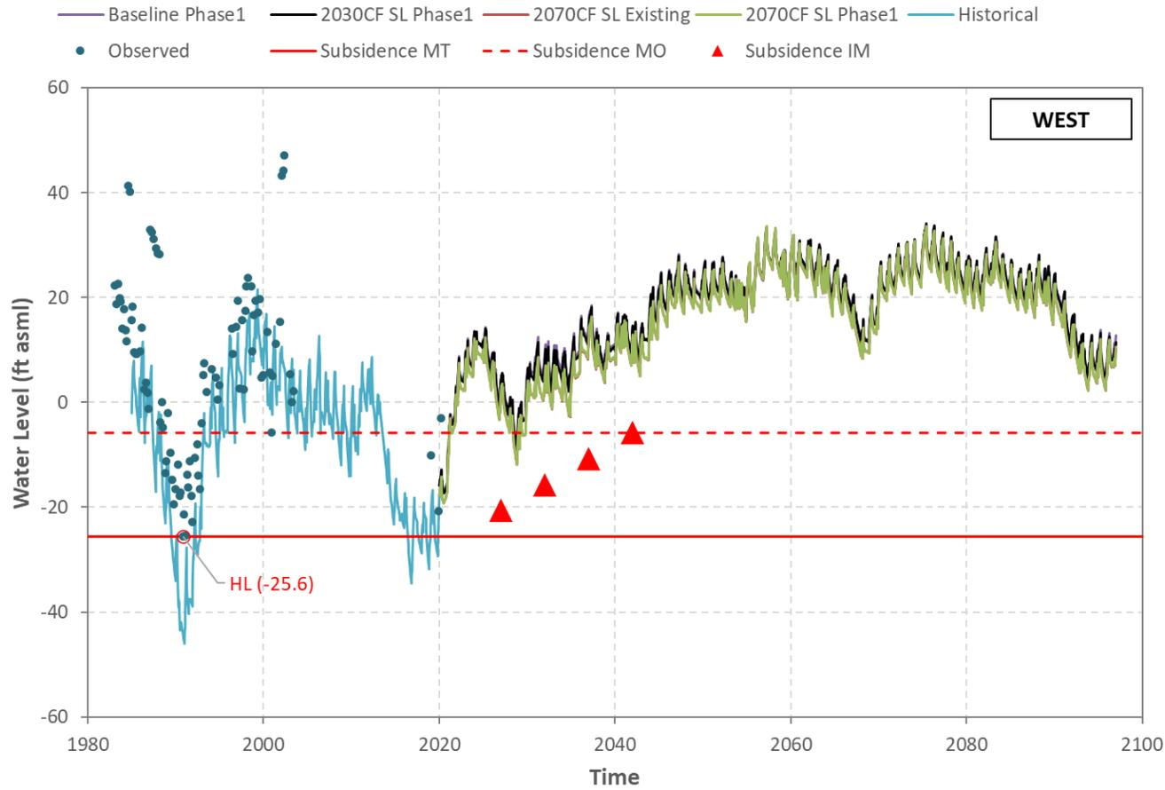
**Figure I-13 Hueneme Aquifer - Simulated/Observed Water Level (Well 02N23W13K04S).**
