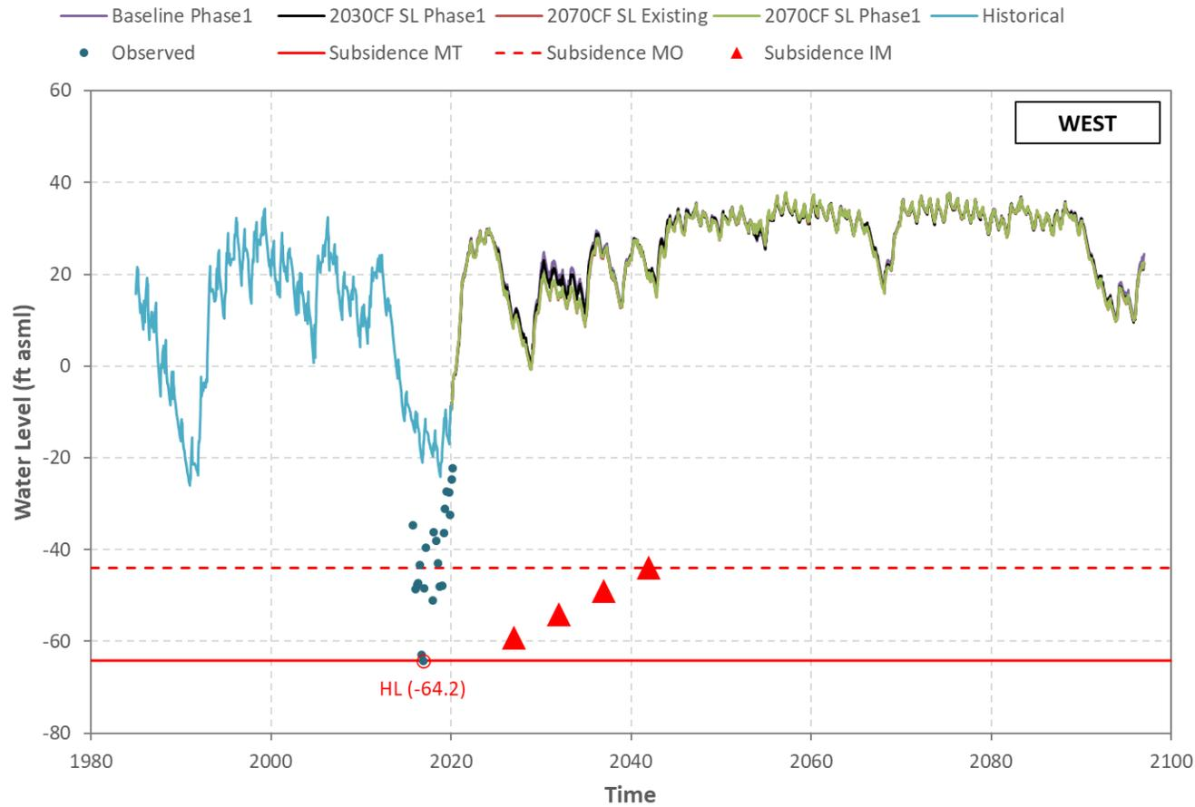
**Figure I-20 Mugu Aquifer - Simulated/Observed Water Level (Well 02N22W19M04S).**
