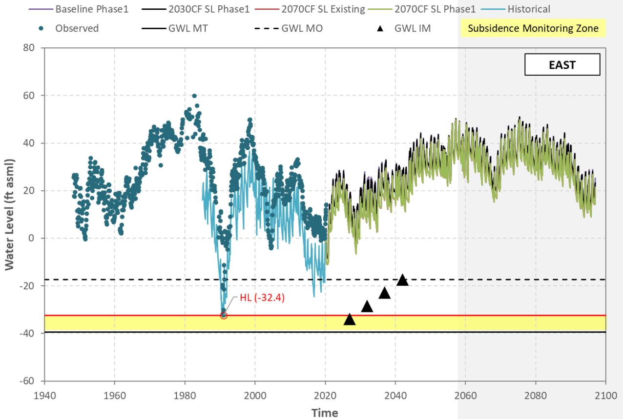
Figure H-2 Hueneme Aquifer - Simulated/Observed Water Level (Well 02N22W09L03S)
