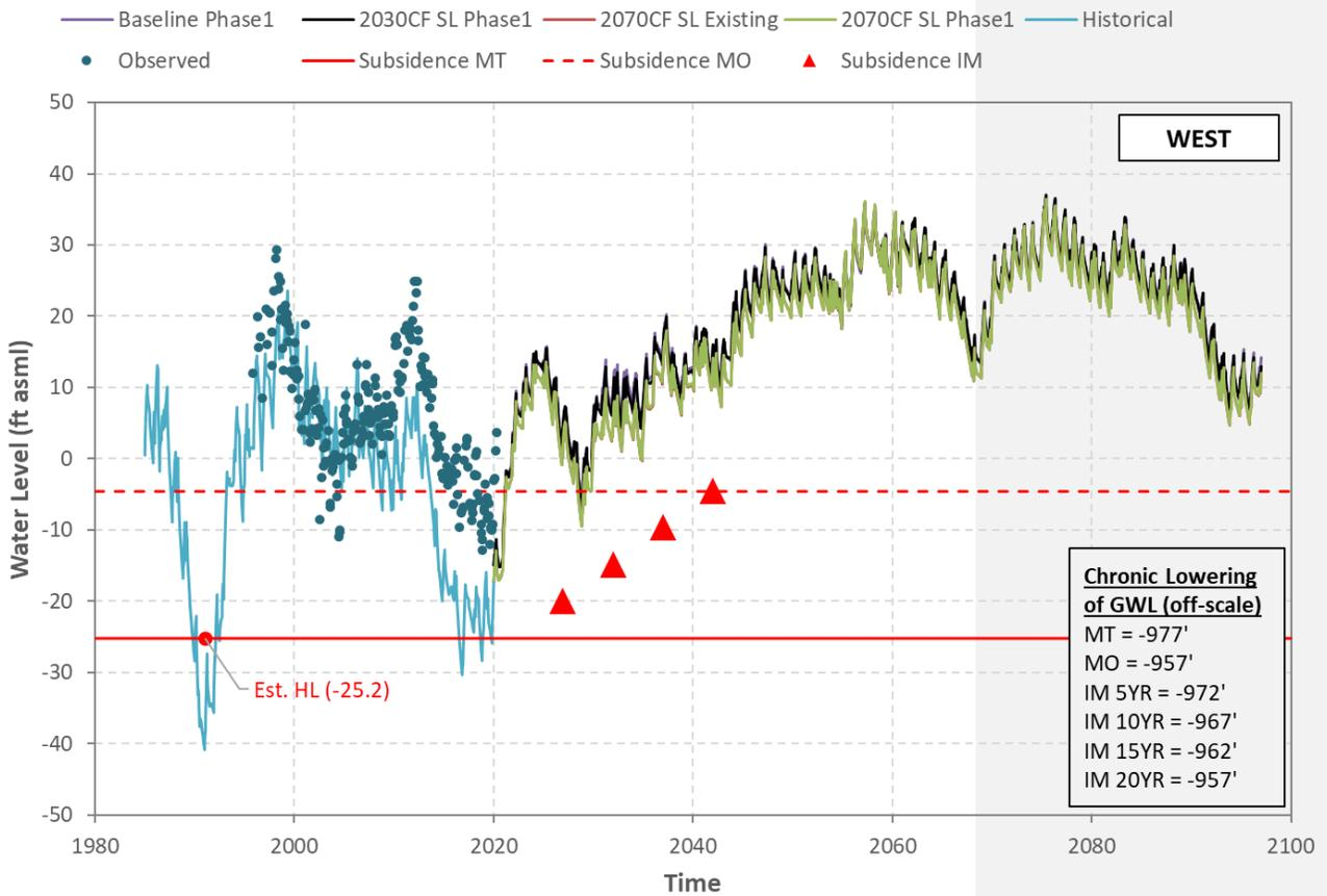
**Figure H-8 Hueneme Aquifer - Simulated/Observed Water Level (Well 02N22W17M02S)**
