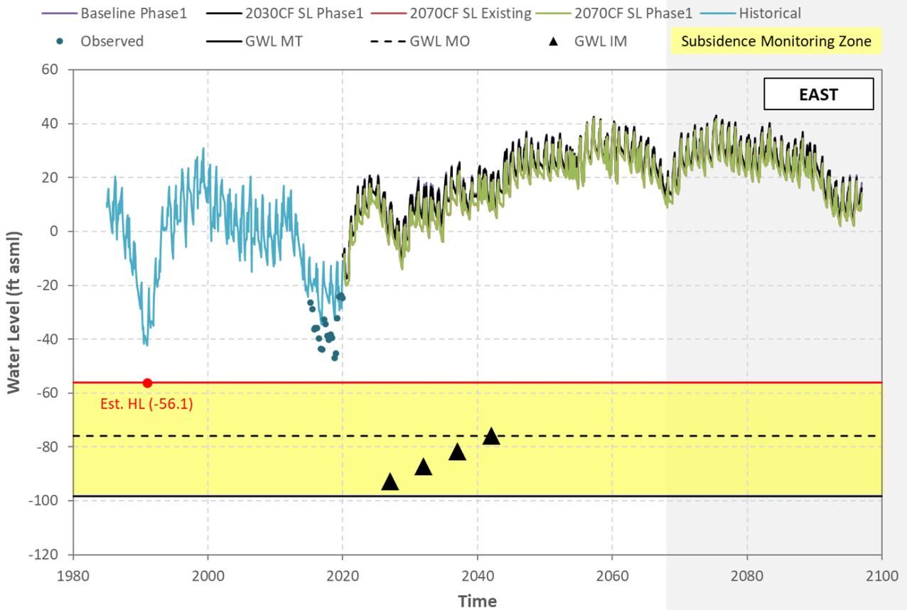
**Figure H-6 Hueneme Aquifer - Simulated/Observed Water Level (Well 02N22W17Q05S)**
