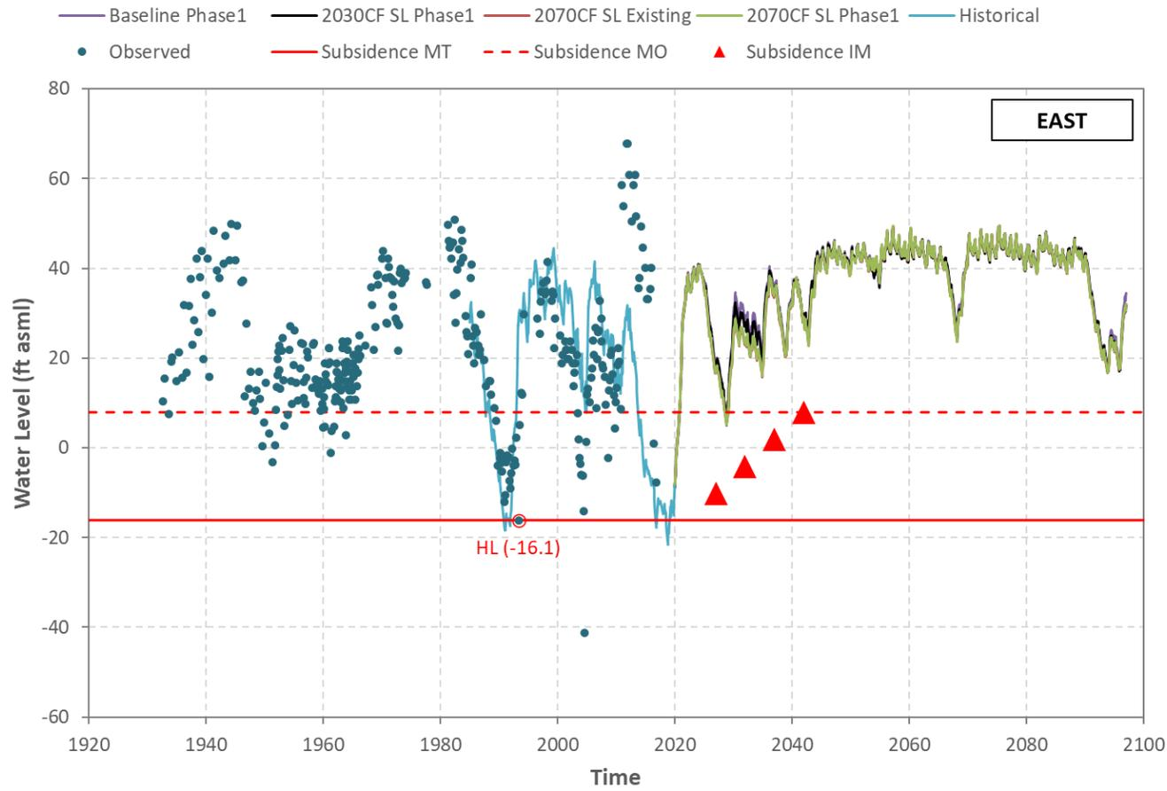
**Figure I-17 Mugu Aquifer - Simulated/Observed Water Level (Well 02N22W08P01S).**
