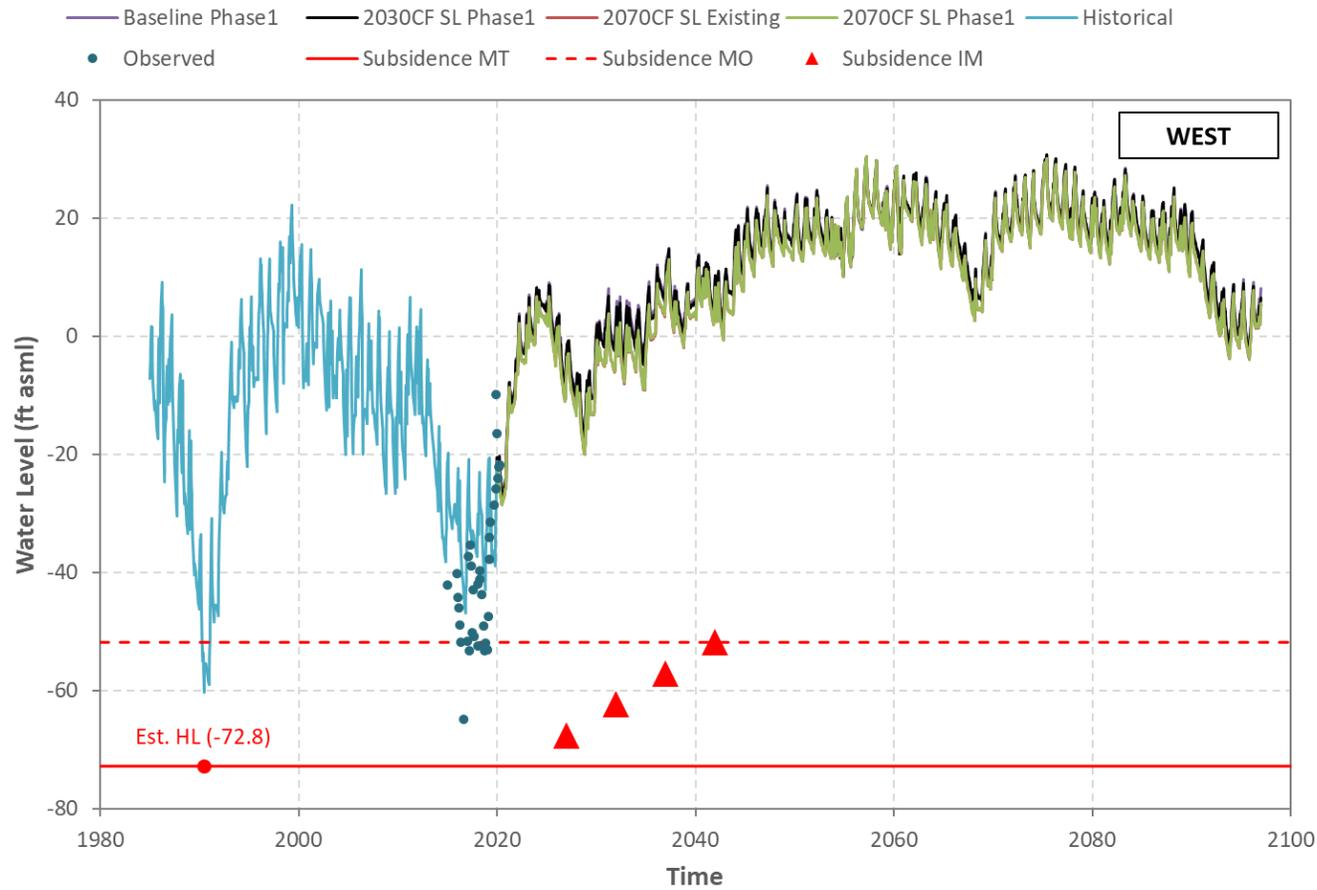
**Figure I-11 Hueneme Aquifer - Simulated/Observed Water Level (Well 02N22W20E01S).**
