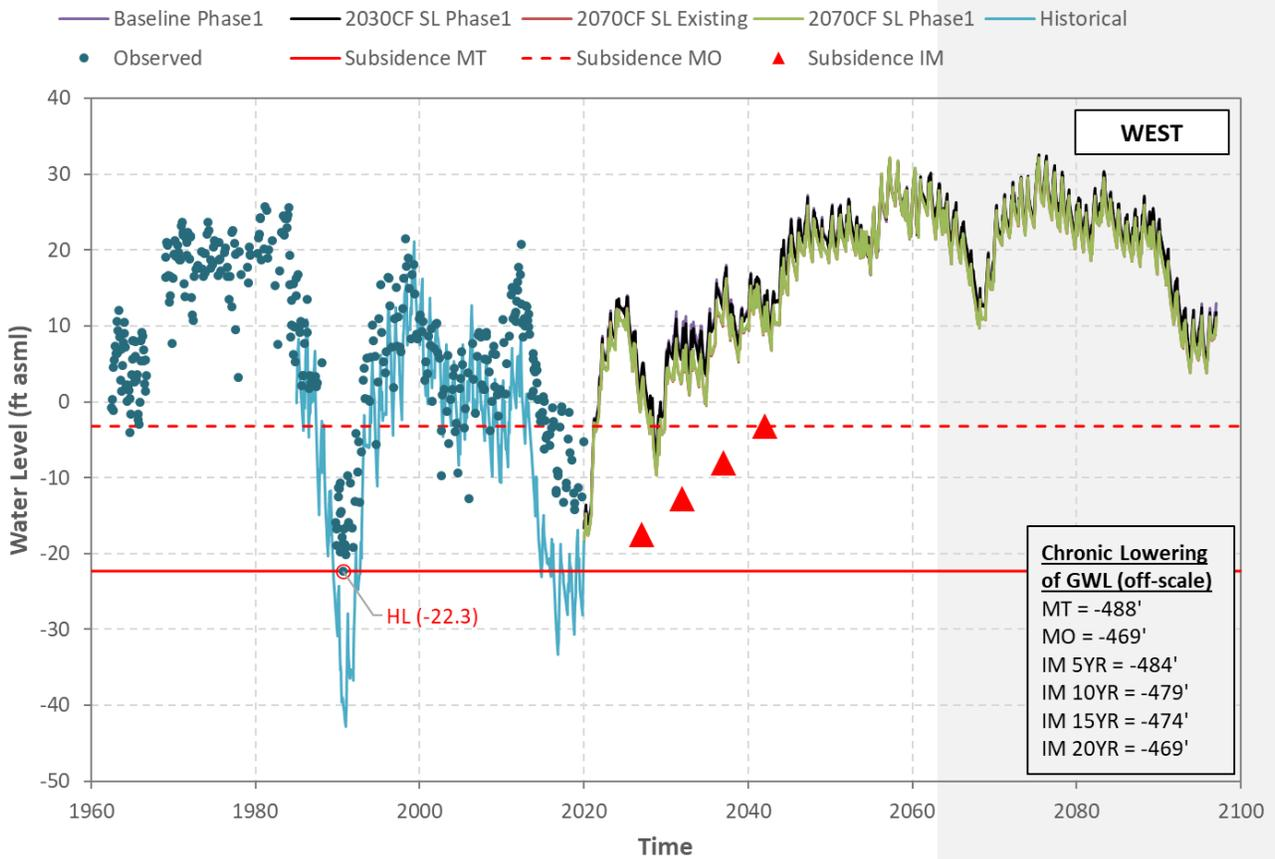
Figure H-14 Mugu Aquifer - Simulated/Observed Water Level (Well 02N22W08G01S)
