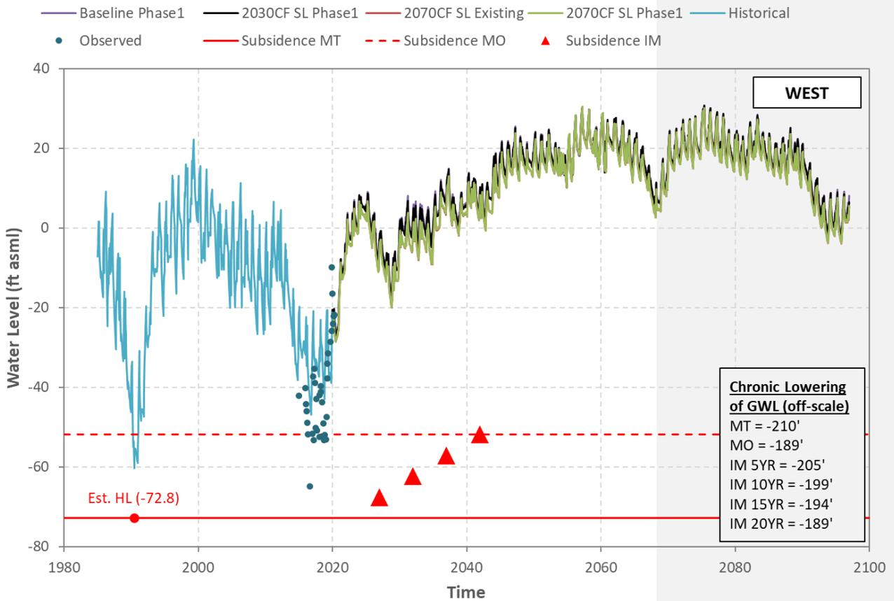
**Figure H-10 Hueneme Aquifer - Simulated/Observed Water Level (Well 02N23W13K03S)**
